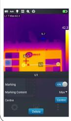
Press and hold any of the analysis objects for a few seconds to display an object menu.
