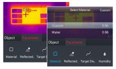
Select **Material** to change measured object's emissivity:
